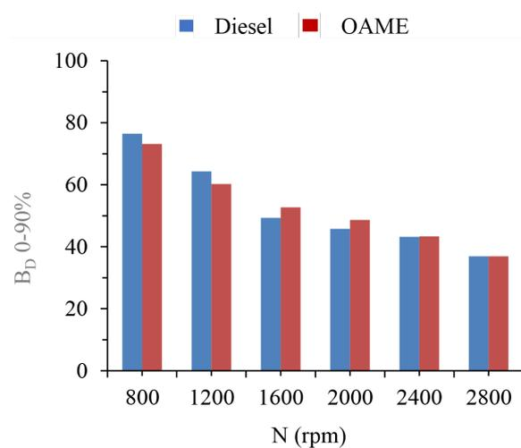
**Figure 11.** Cycle-average burn duration 90% for varied rotational speed
