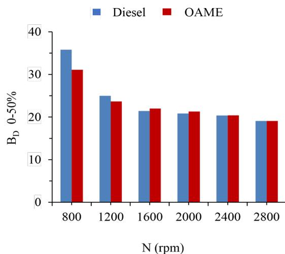
**Figure 10.** Cycle-average burn duration 50% for varied rotational speed
