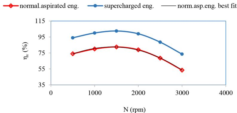
Figure 3. Variation of the volumetric efficiency (Gupta 2012)
