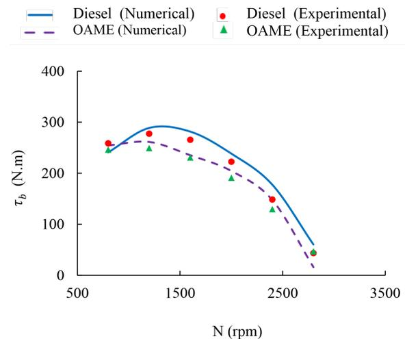
Figure 5. Cycle-average brake torque distribution
