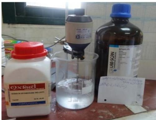
(a) Mixing of catalyst and methanol
