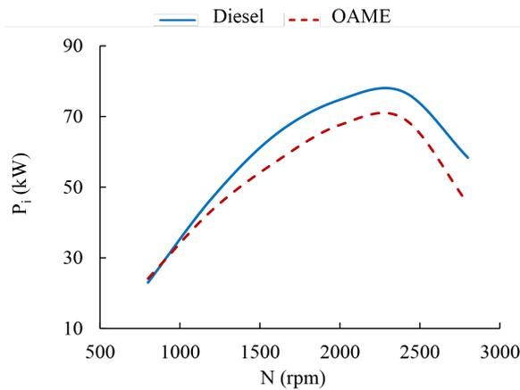
Figure 6. Cycle-average indicated power distribution
