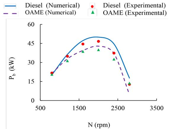
Figure 7. Cycle-average brake power distribution
