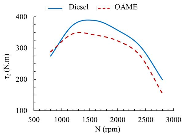
Figure 4. Cycle-average indicated torque distribution
