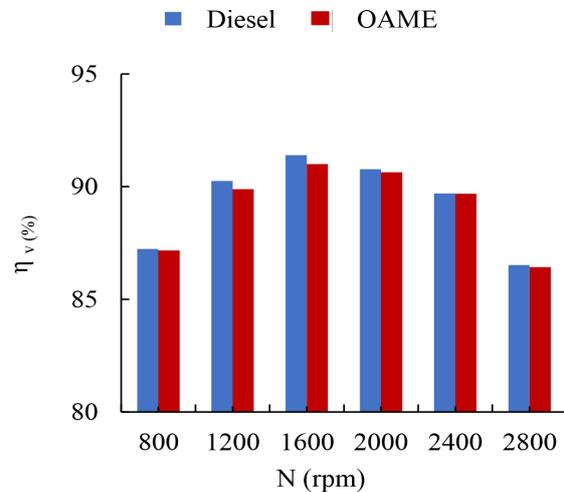
Figure 9. Volumetric efficiency for varied rotational speeds
